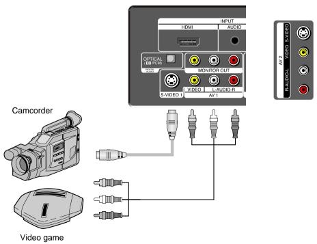
**Note:** If your AV device has both Video OUT terminal and S-Video OUT terminal, S-Video connection is recommended for better picture quality.
